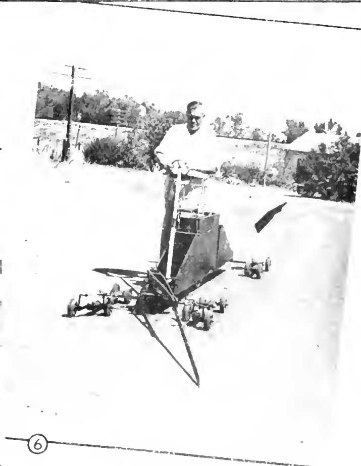
Units of profilograph machine for measuring pavement roughness. 2. Assembling the frame. 3. Close up of recording mechanism. 4. Plan view of the machine. 5. Profilograph assembled, ready for use. 6. Profilograph in use.
